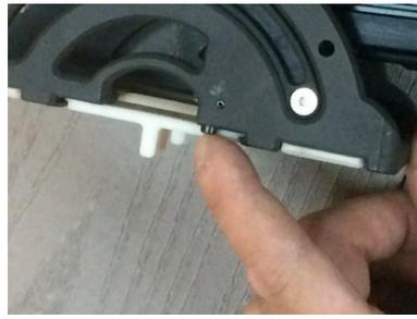
Slide the plate in, and the pin should drop back down by spring pressure. The pin will hold the gap plate in place while the tool is being used. Push the pin in, and slide the plate out when you wish to change plate gap size.
