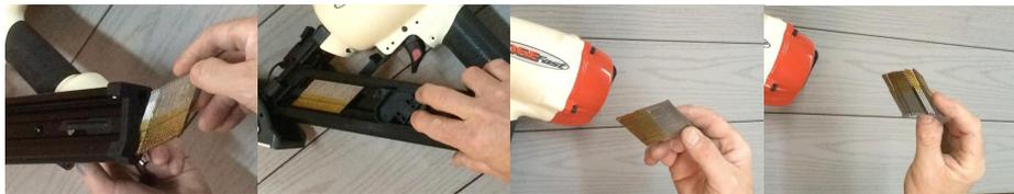
Once fasteners are loaded, then you are ready to engage the spring feed carriage. Push the small button down on the fastener feed carriage, then pull back on the carriage as it rides over the fasteners until it reaches the end of the magazine, and release. Fasteners are now being pushed towards the tool base and driver. Oil the tool each day before connecting air supply, and again after every 1000 shots (3 to 5 drops).
